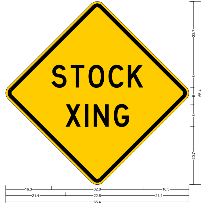
48W11-50; 48.0" across sides 3.0" Radius, 1.3" Border, 0.8" Indent, Black on Yellow; "STOCK", D; "XING", D; Table of letter and object lefts S T O C K 16.3 23.2 29.6 36.7 43.6 X I N G 21.4 28.3 31.4 38.6
