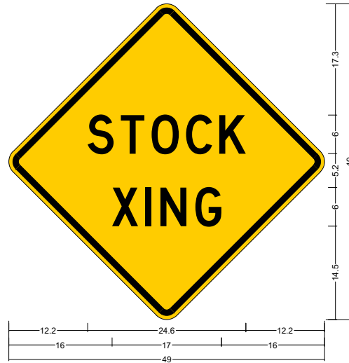
36W11-50; 36.0" across sides 2.3" Radius, 0.9" Border, 0.6" Indent, Black on Yellow; "STOCK", D; "XING", D; Table of letter and object lefts S T O C K 12.2 17.4 22.2 27.5 32.7 X I N G 16.0 21.2 23.5 29.0
